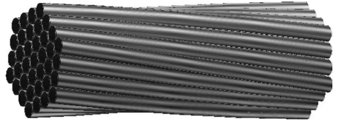
Fig. 1. Schematic showing a stable twisted carbon nanotube rope.
